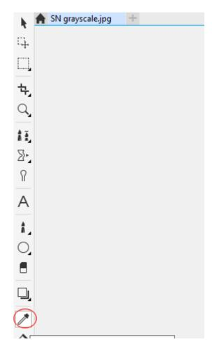
Corel PHOTO-PAINT's **Eyedropper tool**, i.e. the eyedropper tool, tells you the grayscale value of the individual pixels in the image when you move the tool over the image.
