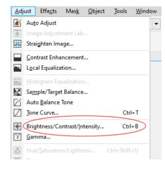
You can roughly adjust the brightness and contrast of the image in the brightness window **Adjust > Brightness/Contrast/Intensity**. The intensity control increases or decreases the total amount of brightness and contrast
